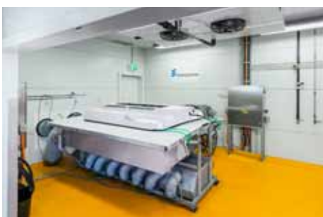
Test chamber for AC system with mechanical compressor
